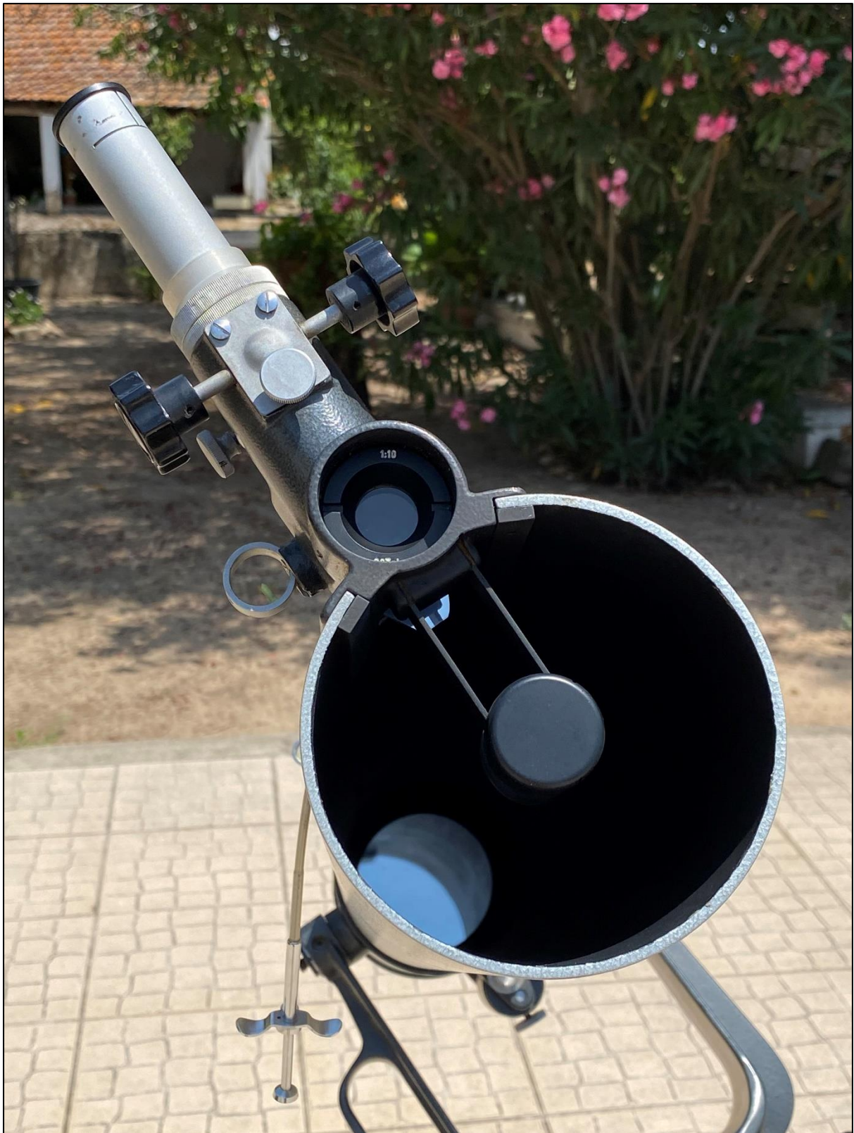
Figure 4 - 20mm finder, 20mm (23.5 mm outside diameter) Huygens eyepiece and main scope.
