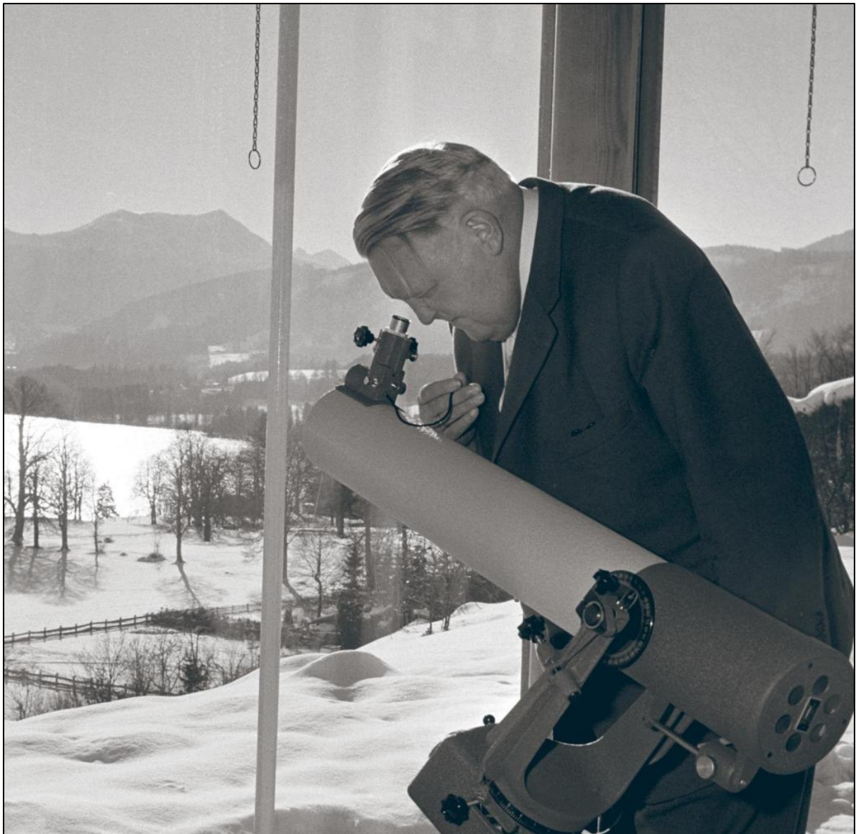
Figure 6 – Ex German chancellor Ludwig Erhard looking through a 100 mm Johannes Heidenhain reflector. Note the mechanism that enables the observer to switch view between the 20mm F/10 finder and the main scope, operated with a cable release.
