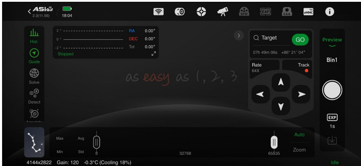
Figure 4 – ASIAIR App. Operates ZWO cameras, auto guiders, filter wheels, and motorized focusers, plus most GoTo mounts.
