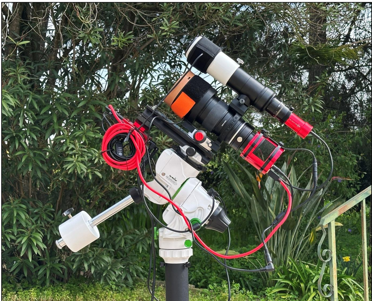
Figure 5 - Samyang 135mm F/2 (@F/2.8), Sky-Watcher Star Adventurer GTi, ZWO ASI AIR Mini, ZWO ASI294MC, ASI120MM Mini (Guide). Pedro RÉ (2025).
